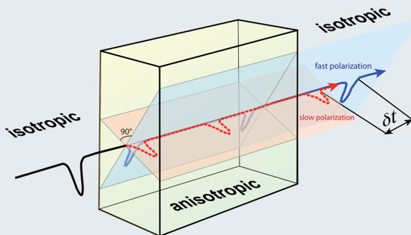
Shear wave splitting in anisotropic media
