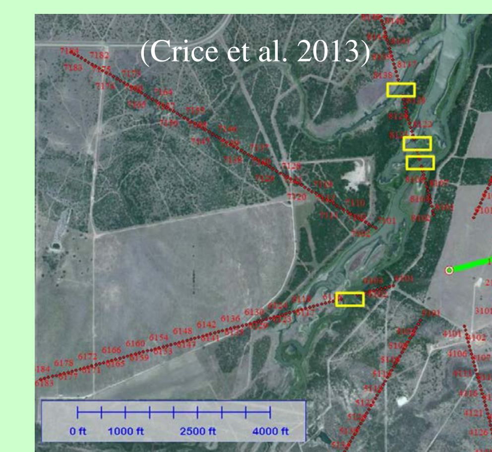
Fig. 5 Surface monitoring challenges. Yellow spots are stream crossings, where it can be difficult to deploy cables
