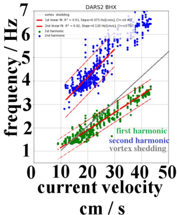
Figure 10: Picked first and second harmonics against the respective current velocity.
