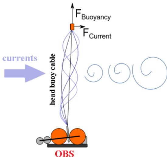
Figure 8: Sketch of strumming head-buoy cable, Stähler et al. 2018
