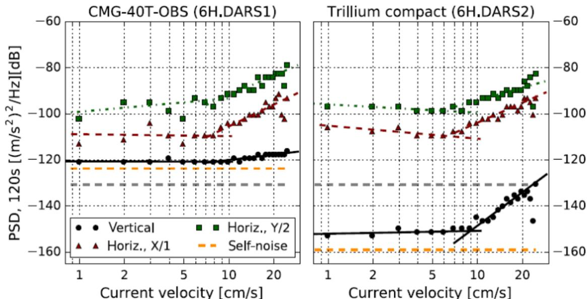
Figure 6: Long periodic (120s) noise levels in relation to prevailing current velocities for CMG-40T-OBS and a Trillium compact.
