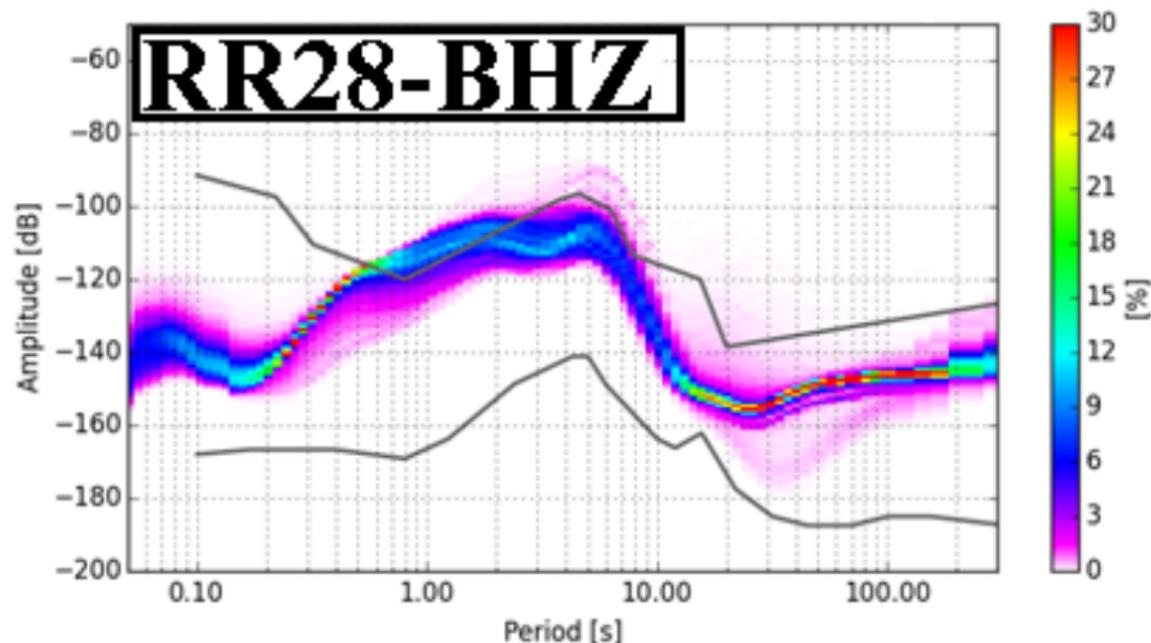
Figure 1: PPSD French of a French OBS
