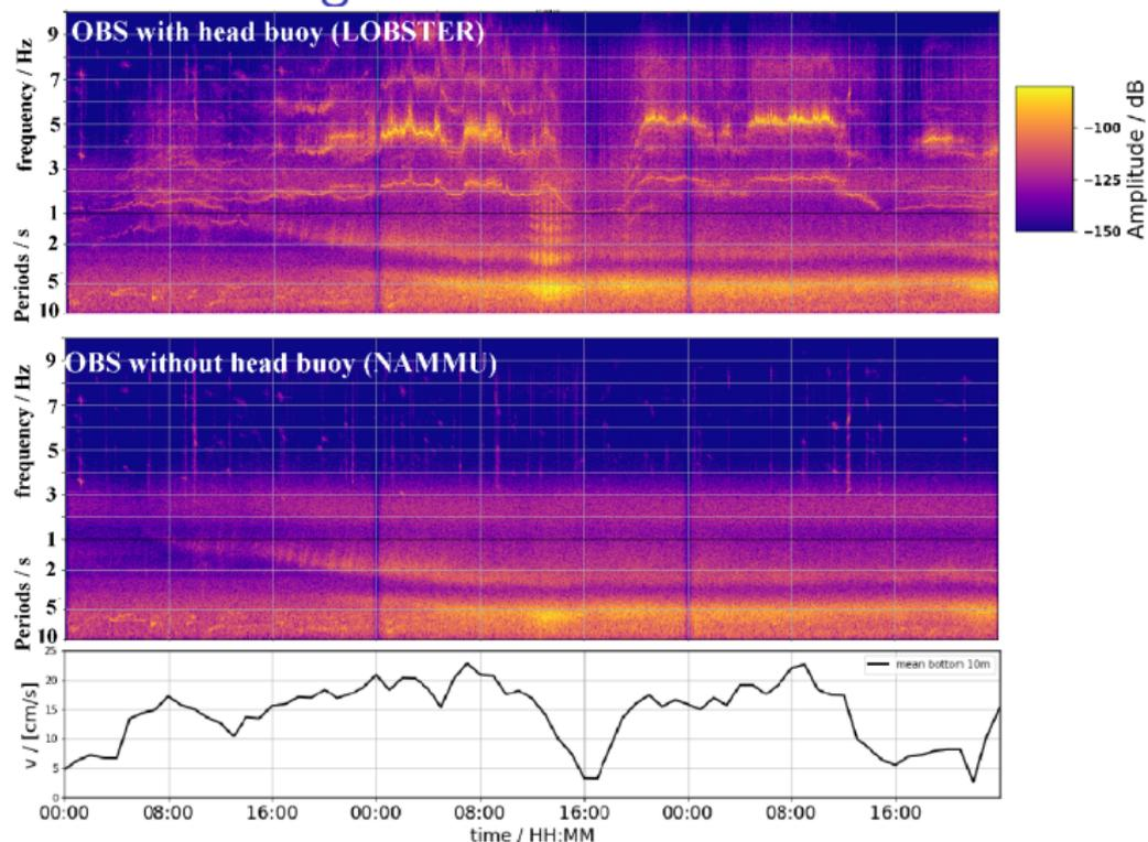
Figure 9: Three day spectrograms of the two different OBS types and measured and averaged bottom current velocities.
