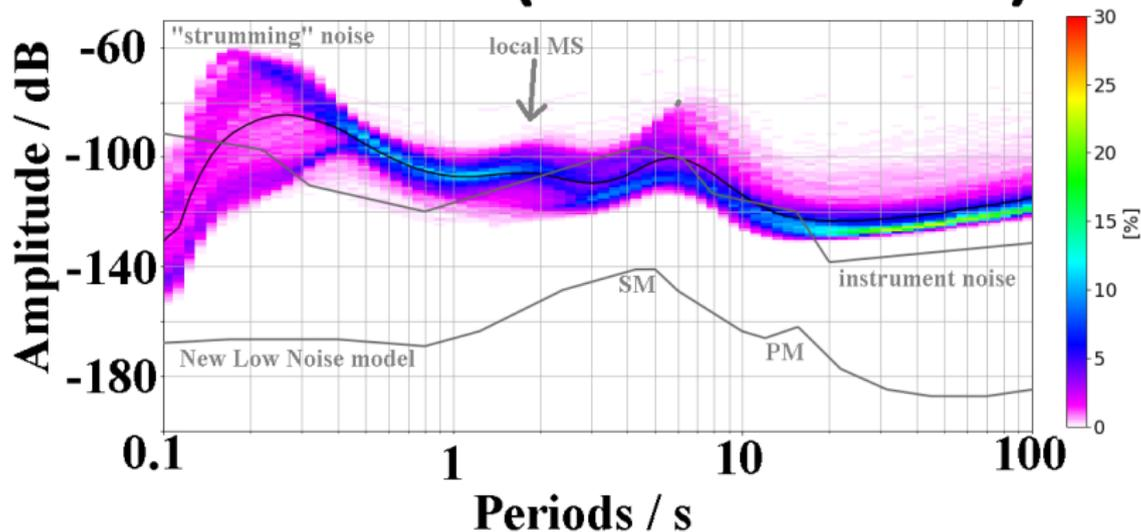
Figure 4: Probabilistic power spectral density plots for the vertical component of the two different seismometer sensors.
