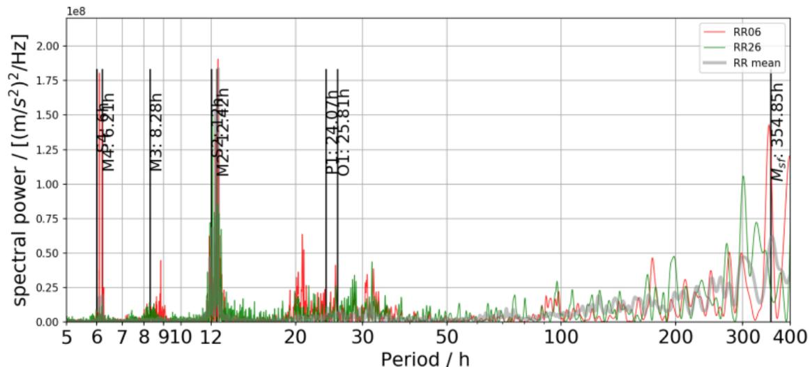
Figure 11: Power spectral density plot for different RHUM-RUM stations shows good agreement with tidal components.
