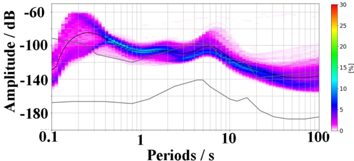
Figure 4: Probabilistic power spectral density plots for the vertical component of the two different seismometer sensors.
